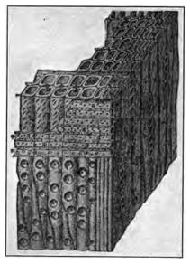
Fig. 26.—Wood of spruce (magnified 100 times). Note the vertical tubes or cells of wood fibers and the bundles of horizontal fibers lying between them.
